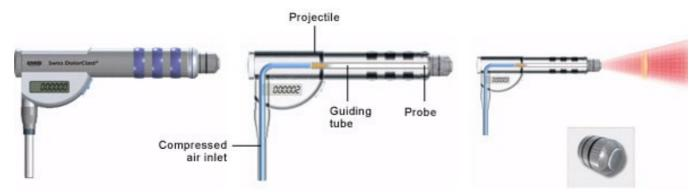
The shockwaves that are produced by the device are generated by a projectile that is propelled at high speed inside a hand-held applicator. When the applicator is placed on the surface of the skin - together with a 'coupling medium' such as ultrasound gel - the impulses are delivered as a shockwave that spreads inside the injured part of the body as a spherical 'radial' wave.
